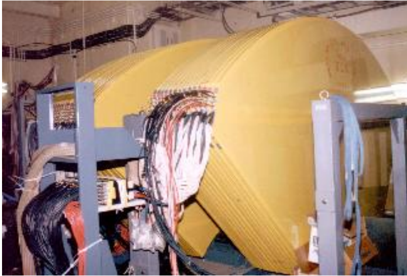
Figure 3.10: Shows the combined iron and tracking components for the endcap portion of the KLM.
