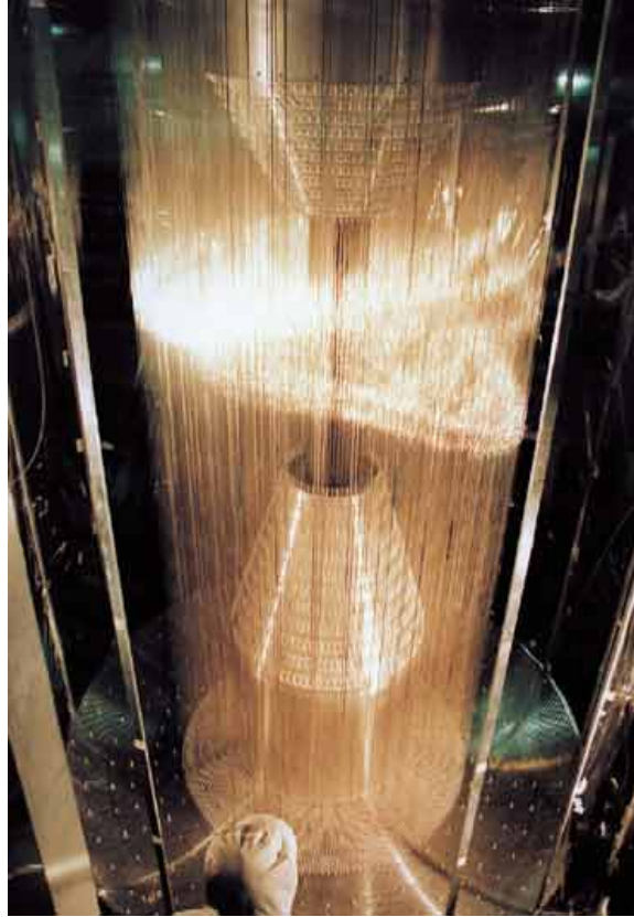
Figure 3.5: Shows the wires of CDC [22].
